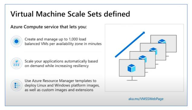
We built a Datacap Web Server VM in the Azure Portal and used this to create a Virtual Machine Scaleset which would scale out (create additional web servers) when the average CPU load exceeds 75% for 5 minutes, scaling in when the average CPU load is less than 25%. There are several available metrics which are adjustable as demands change:
