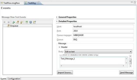
13. After the message has been sent, you can check that it has been sent to OUTQ by looking in Message Broker Explorer and inspecting the queues. You will see a queue depth of 1 on
