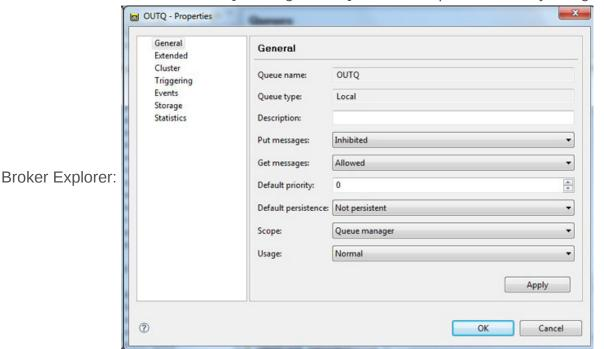
14. Next, test the behaviour of FAILQ. Change OUTQ so that it is put-inhibited by using Message
