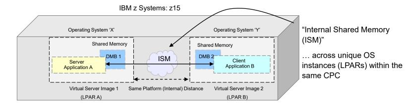
SMC-D (over ISM) extends the value of the Shared Memory Communications architecture by enabling SMC for direct LPAR to LPAR communications. SMC-D is very similar to SMC-R (over RoCE) extending the benefits of SMC-R to same CPC operating system instances without requiring physical resources (RoCE adapters, PCI bandwidth, NIC ports, I/O slots, network resources, 10GbE switches etc.).
