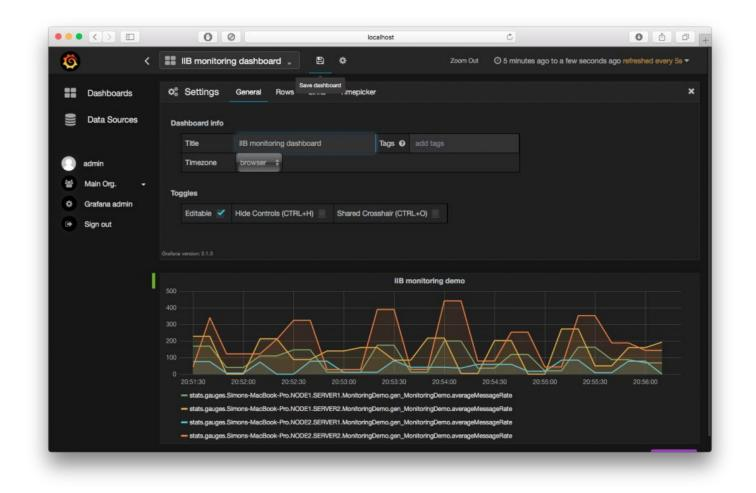
At this point you can monitor the average message rates of message flows across multiple integration nodes and integration servers. You can hover over the graph for specific values for the average message rate at any particular point in the graph:
