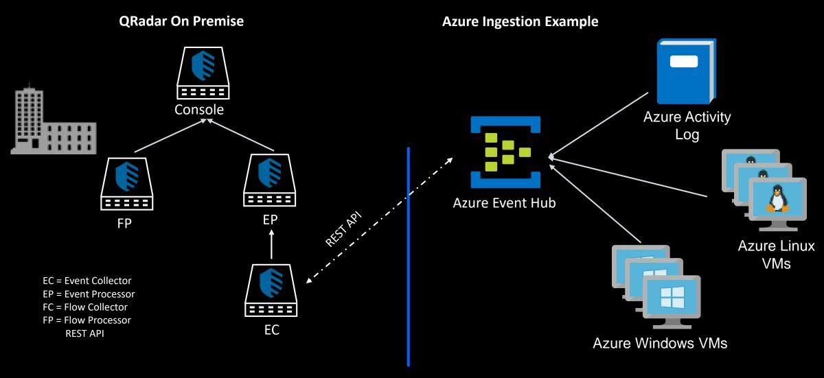
This diagram outlines how event collection works for the Azure Event Hub. Data is sent to the Azure Event Hub and queried by the QRadar On Premise appliance using a REST API.
