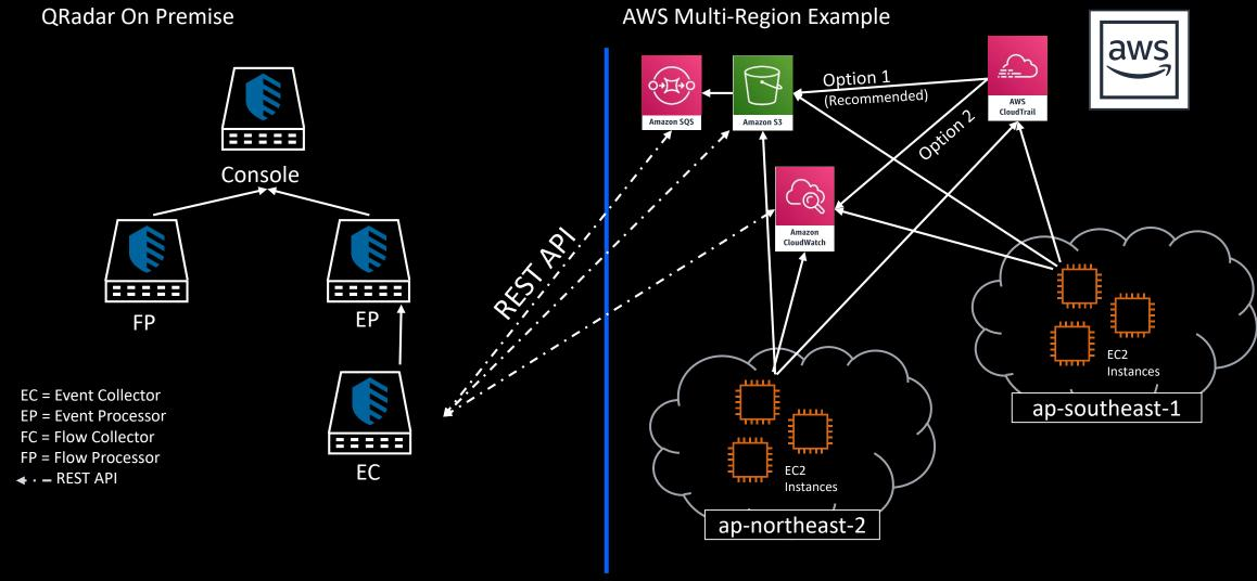
In this architecture outline various data from different AWS Services (CloudTrail, VPC Flow logs, and others) are stored either in S3 or CloudWatch Logs. The QRadar Amazon S3 REST API or AmazonWeb Services Protocols collect this data from the on premise EC or EC/EP combo.
