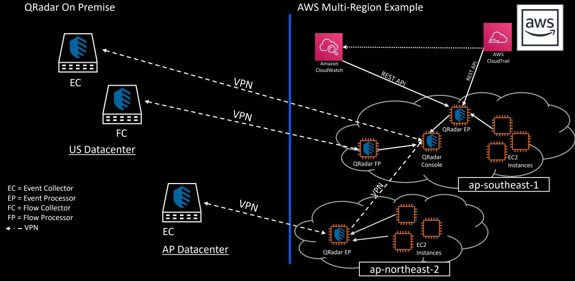
This example outlines on premise Event Collector and Flow Collector appliances that VPN data to the QRadar Cloud deployment. A benefit here is it limits the requirement for HA due to Cloud resiliency.
