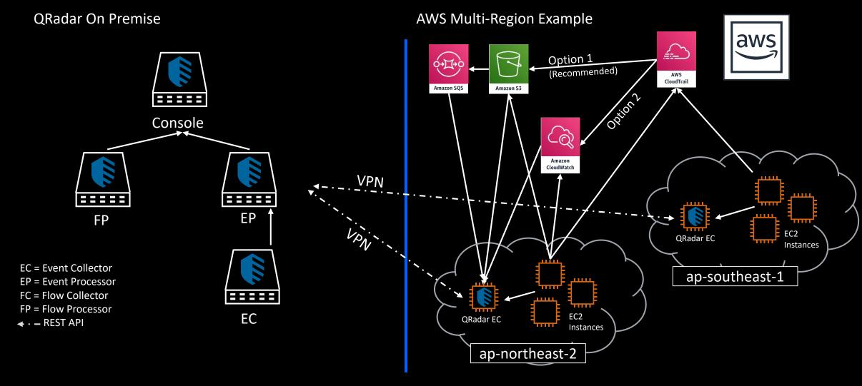
In this architecture outline various data from different AWS Services (CloudTrail, VPC Flow logs, and others) are stored either in S3 or CloudWatch Logs. The QRadar Amazon S3 REST API or Amazon Web Services Protocols collects this data from the CLOUD EC and sends it to an on premise EP. A benefit is that you save on bandwidth as the event pipeline compresses EC to EP connections. Searches are completed with the on premise appliances.
