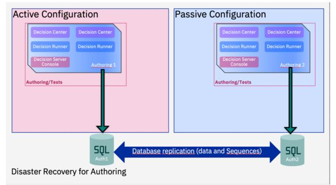
Warning: This architecture is based on the database replication mechanism of data and sequences.
