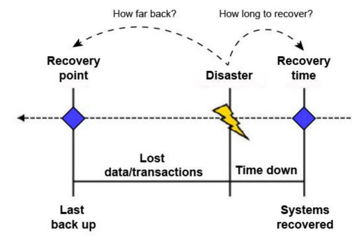
The following diagram shows the relationship between the two measurements:
