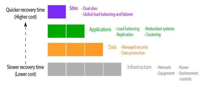
Extreme RTO and RPO goals tend to conflict with one another. For example, using synchronous disk replication of data gives you a zero RPO, but that means the second system can't be operational, which raises RTO.
