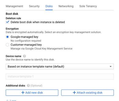
g. When adding disks, you can select which type of disks to add. LSF also supports **Local SSD scratch disk**. Select this from the list of Type.
