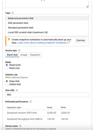
After selecting Local SSD scratch disk, there are two 2 sub-types (SCSI and NVMe). LSF supports both of these, and in the LSF\_TOP/10.1/resource\_connector/google/scripts/user\_data.sh script file, LSF demonstrates a way to automatically mount both kinds of local SSD disks to /tmp.
