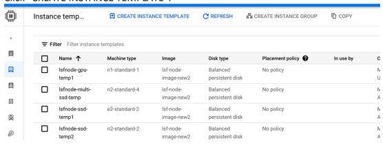
b. Specify a name for the instance template and select the CPU memory and GPU type/number/size for the template by clicking **GPU**, then selecting the GPU type and number for the template.
